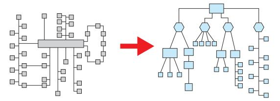
The new anatomy not only helps reduce cost and weight, but also makes it much easier for the different systems in the car (and outside of the car) to cooperate.
