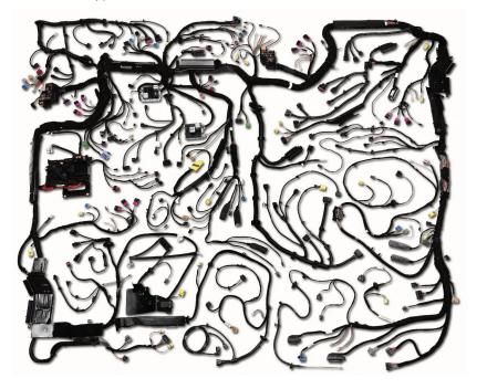
There are multiple proprietary standards for communication in a car, including analog signals on wires, CAN, FlexRay, MOST, and LVDS. Each vehicle component typically has its own dedicated wiring and communication requirements.
