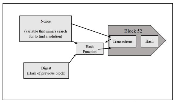
(The diagram above shows the method which the blockchain utilizes to verify and store transactions in block 52)
