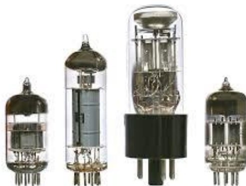
Fig. 2. A set of vacuum tubes that were used in the first ever designed computer systems and the program were hard coded through these vacuum tubes [27] [28]
