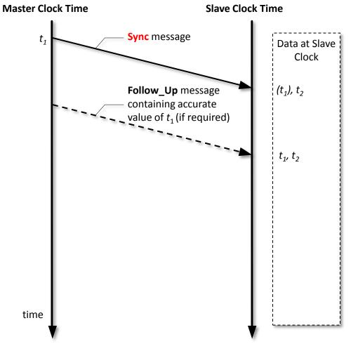
Packet Exchange: Master and Slave exchange time stamped Sync & Delay\_req event messages
